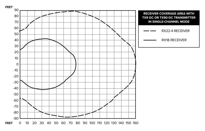
The coverage area for the WIR TX90 DC will vary depending on the receiver being used. The diagram above demonstrates the receiver coverage when operating a single WIR TX90 DC transmitter in single channel mode. Patterns are direct radiation patterns.
